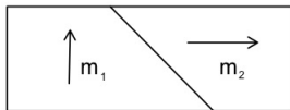
Figure: Div free \mathbf{m} inside domain: \mathbf{m}_1 \cdot \mathbf{n} = \mathbf{m}_2 \cdot \mathbf{n} at transition
